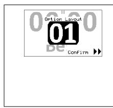
Press Setup to set the maintenance of the lap time, the brightness of the backlight and LED. Each "Layout" is numbered to facilitate the choice, this figure with the word «**Confirm**» appears only a few seconds. Press the button « **Confirm** » to choose, even if this word is no longer visible on the screen.
