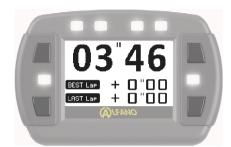
Upon detection of the start line, the system displays window race, timing and recording starts.
